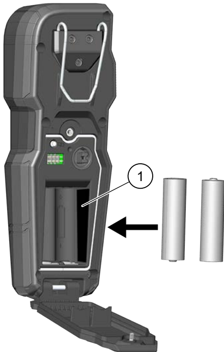
Figure 1. Installing Remote Control Batteries
